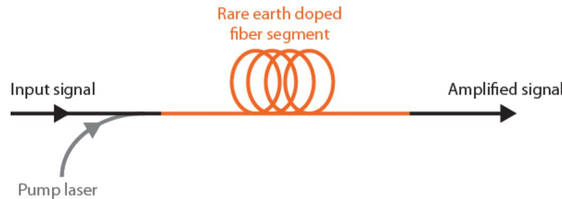
Optically pumped system: energy of pump photons are used to excite atoms
