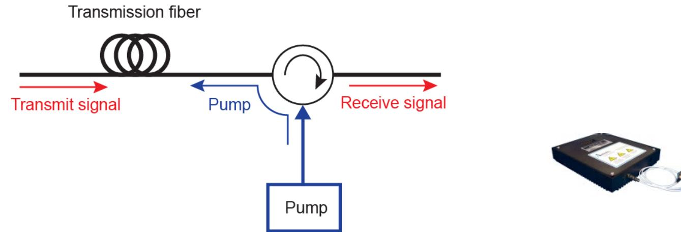
Optically pumped system, uses intrinsic optical nonlinearities of the silica fiber.
